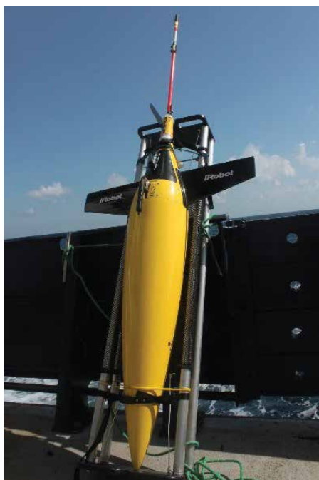
Figure 1: Kongsberg seaglider onboard R/V Sindhu Sathana BoBBLE cruise (2016) during self-tests prior to launch.
