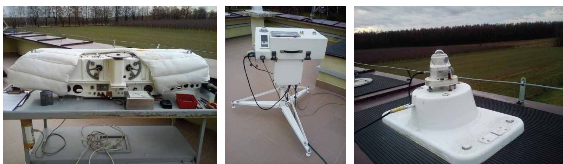
Figure 1: Measuring equipment at the Belsk Observatory. From the left: Dobson spectrophotometer, Brewer spectrophotometer, UV-S-AE-T, Kipp&Zonen meter.
