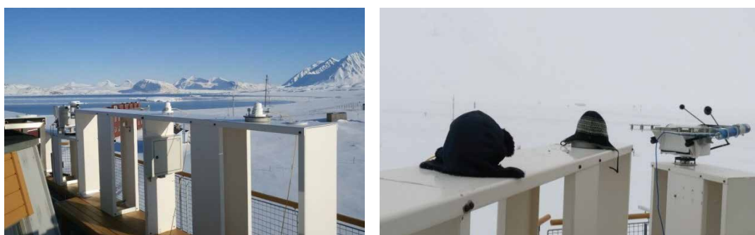
Figure 1: UV meters participating in the UV-ICARE inter-comparison campaign. Instruments, from left to right: UV-RAD, GUV, UVS-E-T of IGF-PAS, UVS-E-T of USB (left). Comparison of the dark current effect by covering the meters with hats (right).
