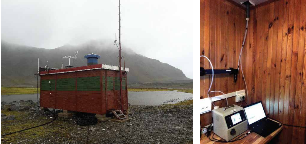
Figure 3: Environmental laboratory in Hornsund. Visible air inlet on the roof (left) and equipment inside (right).
