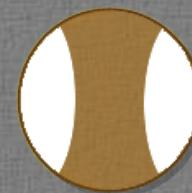
Shear fracture (DC)
