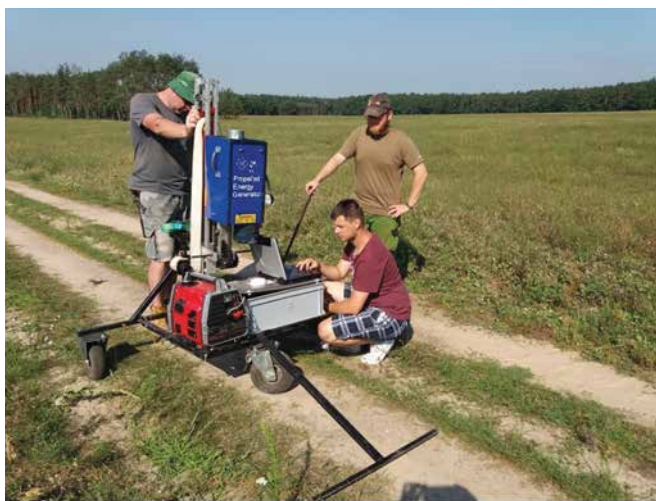
Figure 1 Seismic source PEG-40 adapted to new carriage system, that can be operated without a car. This system can operate in rough terrain like steep hills and dense forest.
