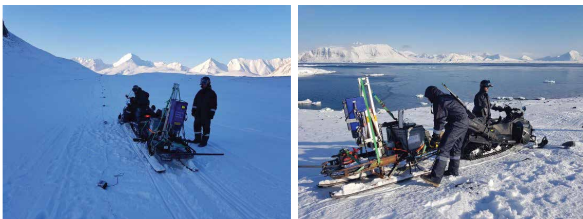
Figure 1 Active seismic team during the field works in Hornsund in April 2018; seismic line composed by DATA-CUBE stations (left), seismic source PEG-40 mounted on sledges (right).
