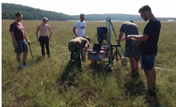
Figure 1 Outdoor training at the profile Mosty 1. Assembling of enhanced PEG-40 seismic source.
