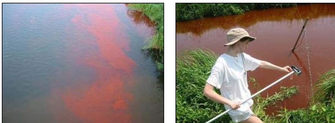
Figure 5. Spreading of fluorescent dye a) at the early stage where 3D mixing occurred and b) at the stage where the tracer was mixed across the entire cross-section.
