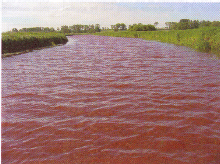
Fig.3. The view of the Narew River at a long distance from the release point, i.e. at the stage where the tracer is mixed across the entire cross-section.
