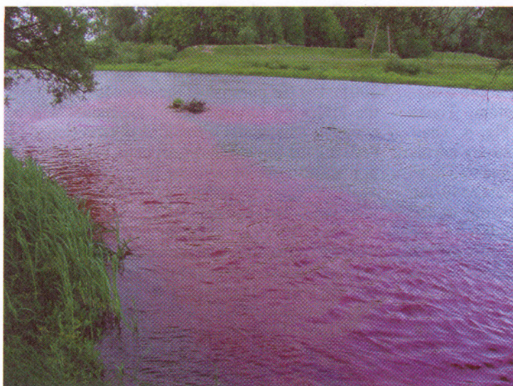
Fig.2. Spreading of Rhodamine WT at the early stage where lateral mixing occurs.
