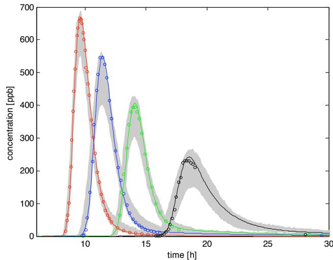
Figure 3.1: Comparison of observed (dots) and simulated (solid line) concentrations of Rhodamine WT at cross-section 3N, 5N, 6N and 7N with 95% confidence bounds
