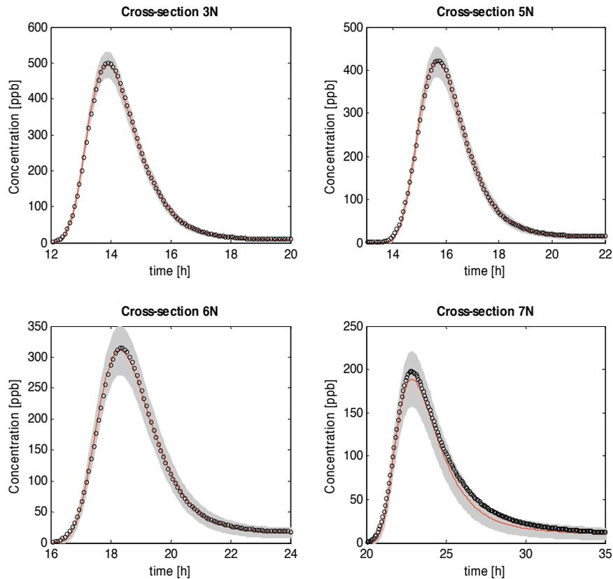
Figure 5.1: Validation of active mixing volume model. Open circles represent virtual reality simulated by mechanistic model, red solid line – ADZ model; shaded areas show 95% confidence bounds obtained from the ADZ model.
