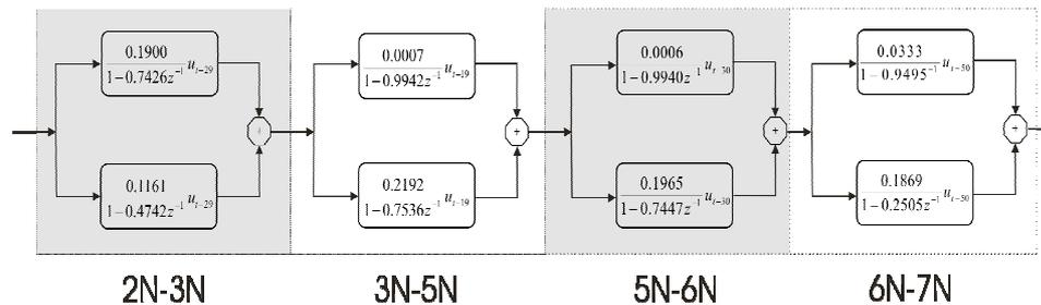
Figure 4.1: Transfer function block diagram of the whole analyzed river reach model
