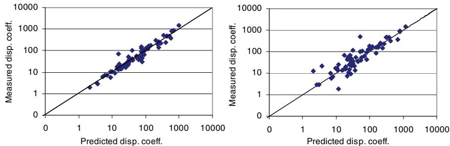
Figure 2. Comparison of ADE longitudinal dispersion parameter fitted to measurements and evaluated from multi-layer perceptron neural network when sinuosity index is considered (left) or when it is not considered (right) – logarithmic scale.
