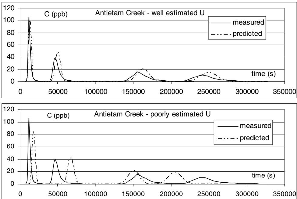
Figure 4. Predicted and measured breakthrough curves for Antietam Creek (USA) for which little information is available.
