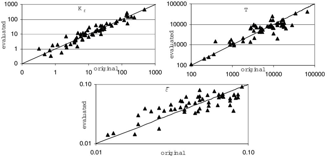
Figure 1. Comparison of TSM parameters fitted to measurements and evaluated from multi-layer perceptron neural network – logarithmic scale (after Rowinski and Piotrowski, 2008).
