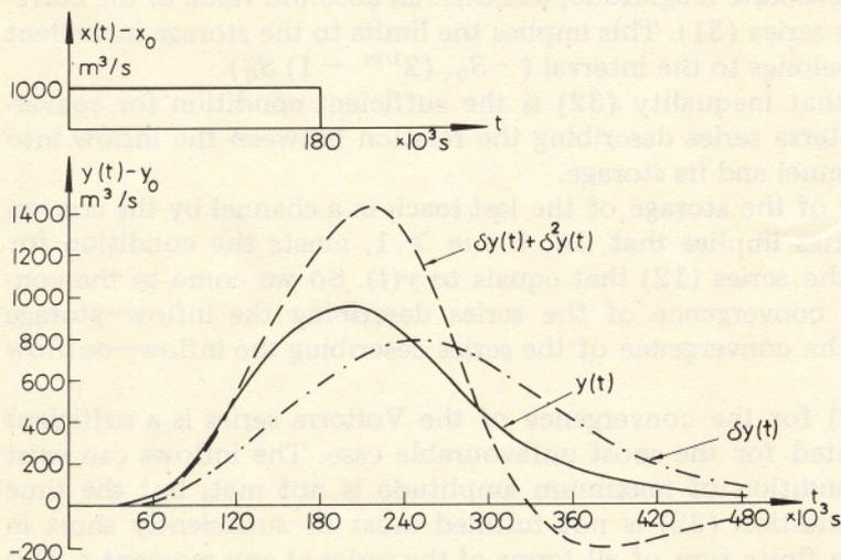
Fig. 4. Comparison of the results of simulation of the outflow by the first  $\delta y(t)$  and the first two terms  $\delta y(t) + \delta^2 y(t)$  of the Volterra series in the case when condition (32) is not met.
