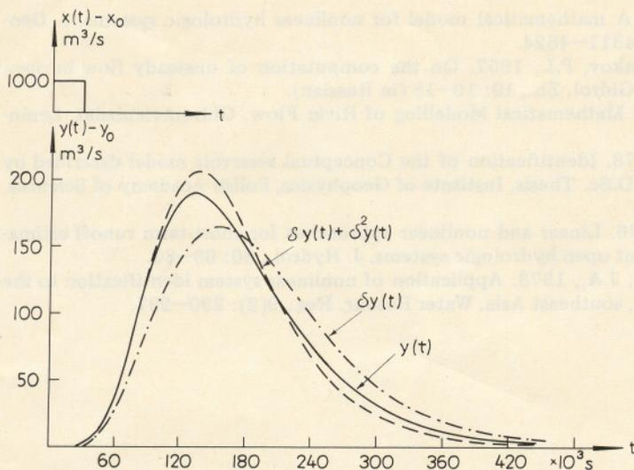
Fig. 5. Comparison of the results of simulation of the outflow by the first  $\delta y(t)$  and the first two terms  $\delta y(t) + \delta^2 y(t)$  of the Volterra series in the case when condition (32) is not met but the series converges.
