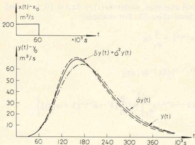
Fig. 3. Comparison of the results of simulation of the outflow by the first  $\delta y(t)$  and the first two terms  $\delta y(t) + \delta^2 y(t)$  of the Volterra series provided condition (32) is met.
