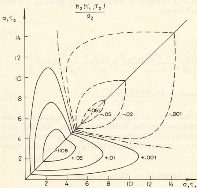
Fig. 2. The second-order kernel of the Volterra series describing five reaches of a channel.
