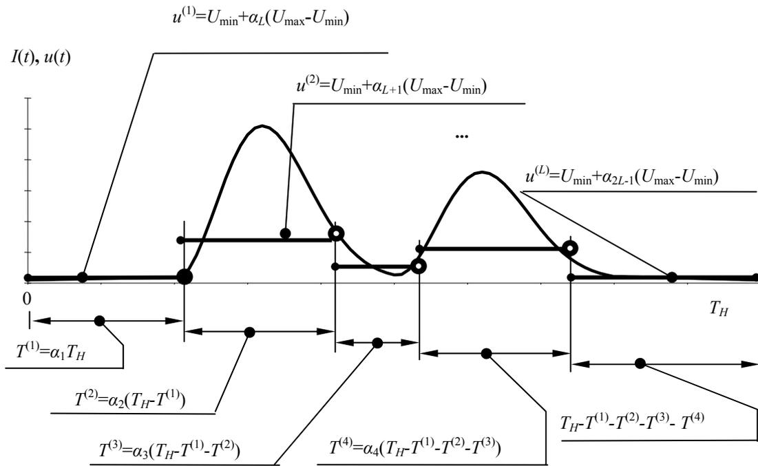
Fig. 4. Control functions as a train of rectangular pulses.
