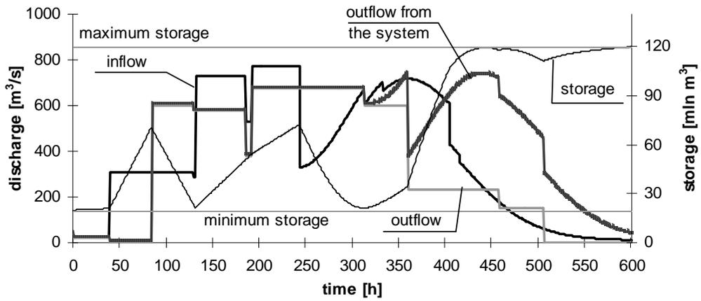
Fig. 6 (d). Trajectories of inflow, outflow and storage for the fourth reservoir.
