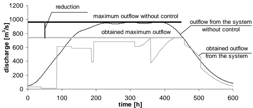
Fig. 6 (e). Comparison of the uncontrolled outflow from the reservoirs with that obtained by means of CRS method.
