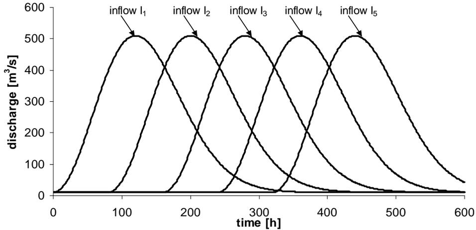
Fig. 5. Inflow hydrographs to the system of four reservoirs in series.
