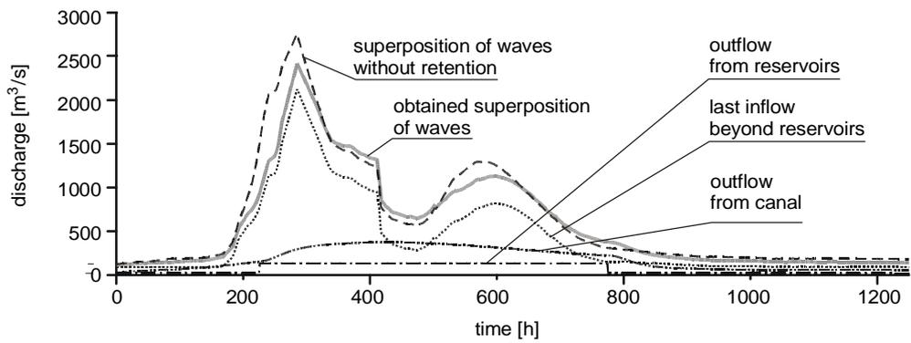
Fig.7 (c). Flow at the cross-section below the junction of Nysa and Odra Rivers.
