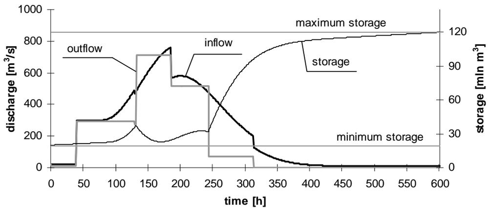
Fig. 6 (b). Trajectories of inflow, outflow and storage for the second reservoir.
