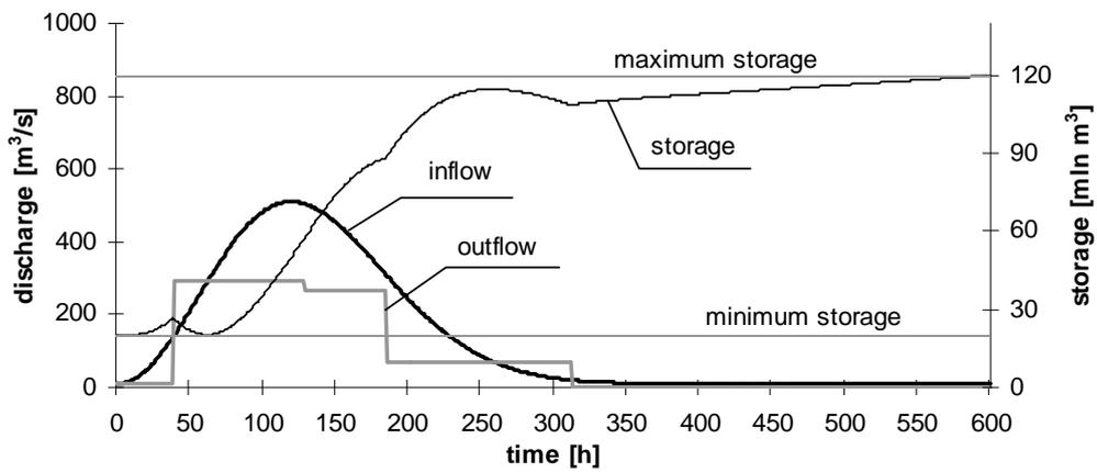
Fig. 6 (a). Trajectories of inflow, outflow and storage for the first reservoir.
