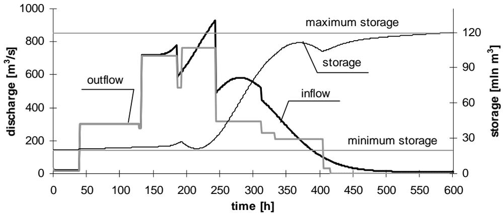
Fig. 6 (c). Trajectories of inflow, outflow and storage for the third reservoir.
