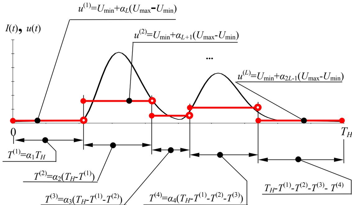
Fig. 2 Control functions as a train of rectangular pulses
