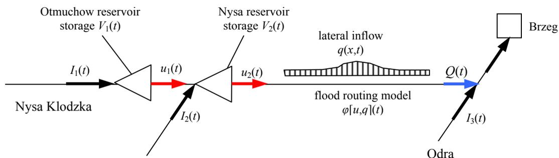
Fig. 1 Schematic representation of the system
